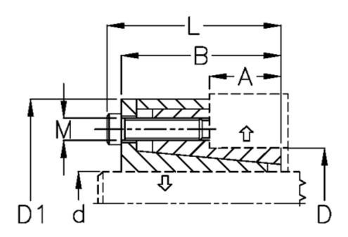
A mm = 27 B mm = 46.0 D1 mm = 57.0 d H8 mm = 24 D mm = 38 F kN torque = 34 L mm = 52.0 M mm = 6 P N/mm2 surface pressure on shaft/hub = 81
